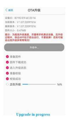
The overall upgrade time takes  $1\sim3$  minutes. The upgrade must be done within 3m of the module, otherwise the upgrade will fail due to poor Bluetooth signal.
