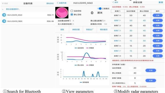
The process of modifying the radar parameters of the Bluetooth APP is the same as that of the PC host computer tool.
