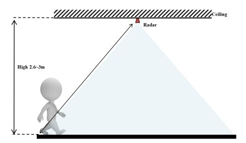
Figure 7 Schematic diagram of ceiling-mounted installation
