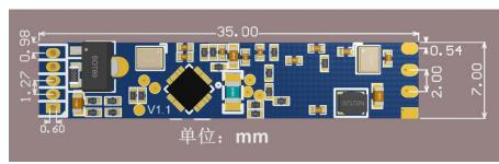
**Figure 5 Module Dimensions**
