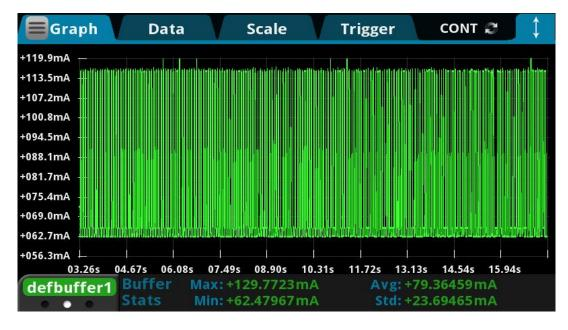
Figure 11 Measured data of module working current
