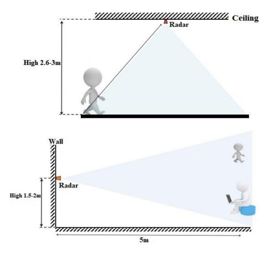
Figure 1 Diagram of usage
