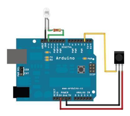
Then we'll write a sketch which will pulse pin #13 on and off very fast in the proper code sequence.
