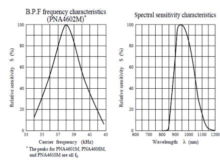
As you can see from these datasheet graphs, the peak frequency detection is at **38 KHz** and the peak LED color is **940** nm. You can use from about 35 KHz to 41 KHz but the sensitivity will drop off so that it wont detect as well from afar. Likewise, you can use 850 to 1100 nm LEDs but they wont work as well as 900 to 1000nm so make sure to get matching LEDs! Check the datasheet for your IR LED to verify the wavelength.
