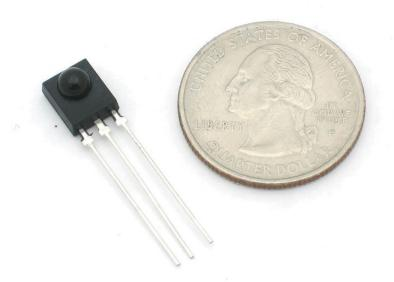
IR detectors are little microchips with a photocell that are tuned to listen to infrared light. They are almost always used for remote control detection - every TV and DVD player has one of these in the front to listen for the IR signal from the clicker. Inside the remote control is a matching IR LED, which emits IR pulses to tell the TV to turn on, off or change channels. IR light is not visible to the human eye, which means it takes a little more work to test a setup.
