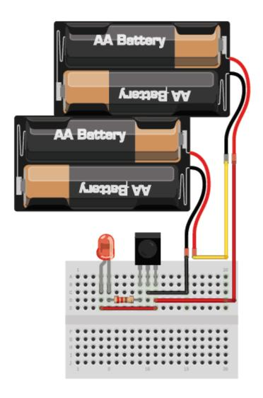
We will use 4xAA 1.3V batteries (I use NiMH) so that the voltage powering the sensor is about 4V.
